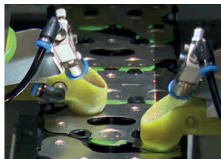
Tab welding on battery cells
