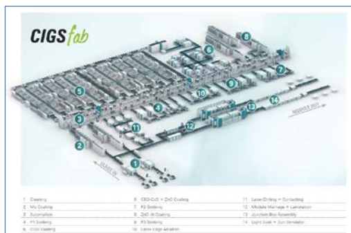
Image 3: Layout of a Manz CIGSfab, just like the one currently under development in Chongqing. Through its global production network, the German high-tech equipment manufacturer is able to cover all of the essential steps required to produce CIGS thin-film solar modules on glass substrates.
