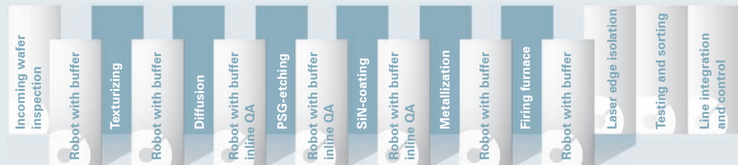
Crystalline solar cells production line process stages
